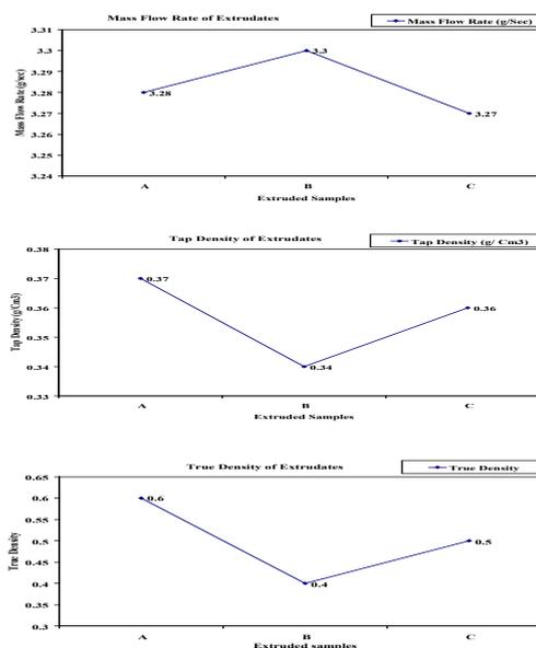
**Figure 1.** Mass flow rate, tap density and true density of extrudates
